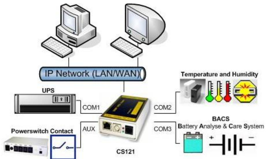
CS121 (not Budget) production after 04/2007 is equipped with an enhanced AUX port („COM3“) which also allows to connect a **BACS (Battery Analyse & Care System)** to the CS121.
