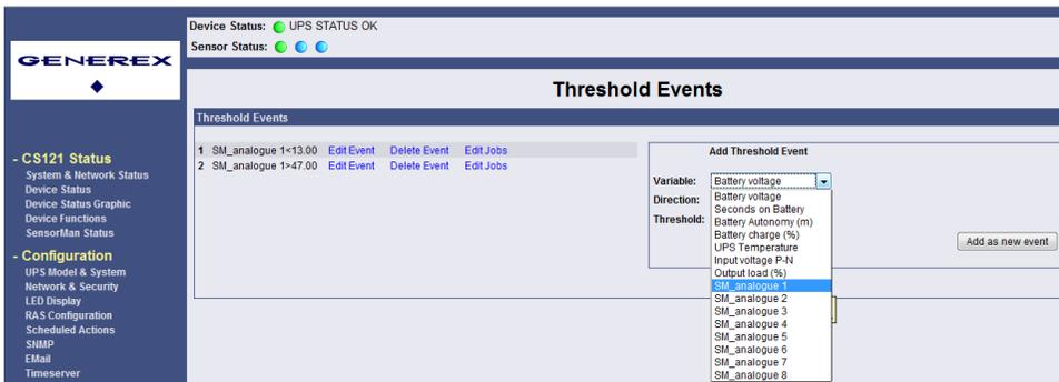
Figure 101: CS121-Configuration Threshold Events of analogue Inputs
