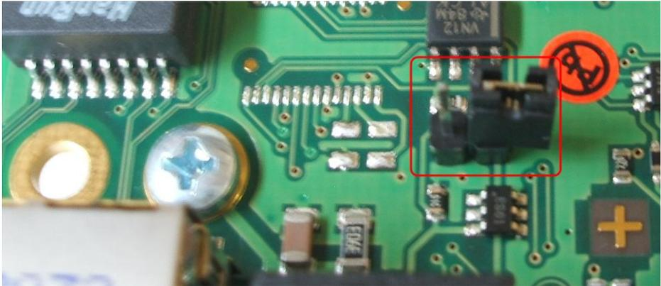
Figure 150: MODBUS - Jumper
