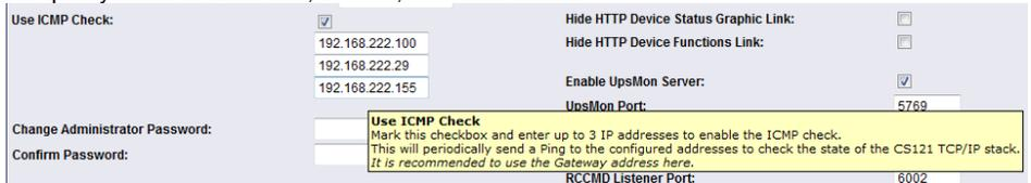
Figure 19: HTTP - Network & Security ICMP Check
