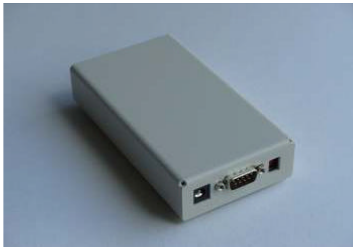
CS121 BL, external aluminum chassis, type label with serial number starting: "0121B"
