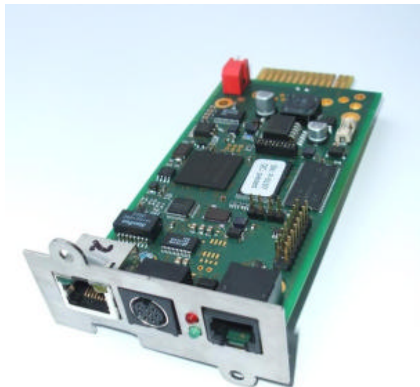
CS121 SC (HW131), PCB slot view, front side
