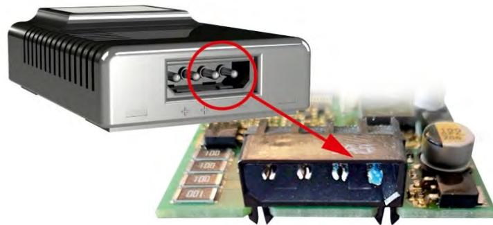
**Our investigations have shown that the BACS modules (and all connecting cables) were contaminated with a basic electrolyte.**
