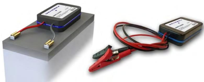
*Picture: SMARTLOGGER with FASTON 6.3mm (also available with ring cable lugs in various sizes and lengths) and SMART LOGGER with “crocodile clips” for battery service technicians to record data during a capacity test of UPS batteries.*
