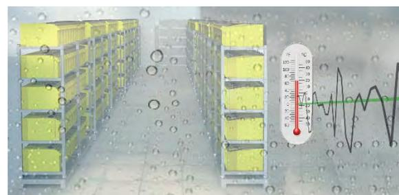
The result of condensation in potentially contaminated rooms (sulphur, salt crystals) creates an aggressive atmosphere and thus corrosion on all exposed parts, including in long-term operation on parts protected by protective varnish. This sometimes led to the complete failure of the modules and cables used.
