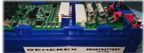
*Picture: SMARTBATTERY (in blue) with integrated SMARTLOGGER, high-voltage fuses and interface (an 8-pin connector) to the “iBACS” BACS module for optional insertion into the SMARTBATTERY.*
