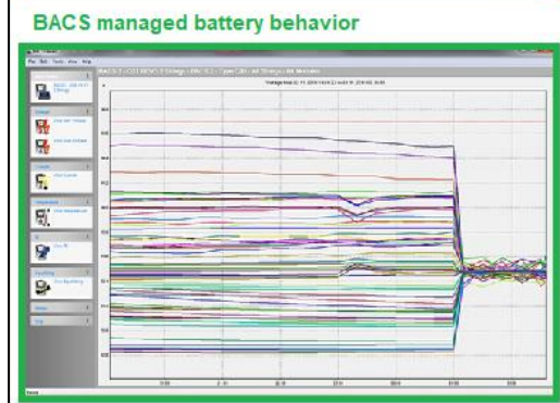
BACS® VIEWER SCREENSHOT As seen by BACS®, the same 5-year-old system as shown in the previous graphic, this time, after the application of the genuine Equalization (Balancing) process. Within a few hours, this process brings the variance in float voltage to within 1/100th of a volt of the level recommended by the
