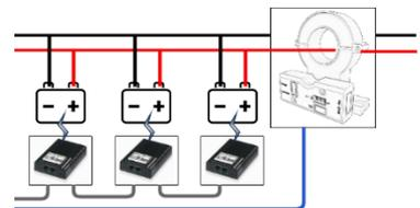
***BACS - Ground fault mode wiring (CSHxxx D only)***
