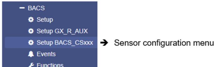
Check the box at „BACS CS Current Sensor Connected“ to enable the sensor
