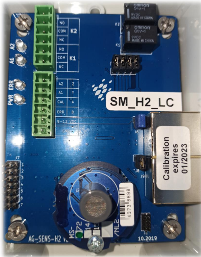
Board layout of the SM_H2_LC standard sensor device
