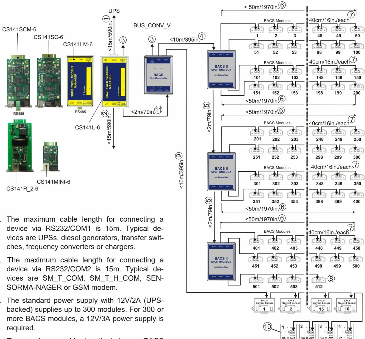
1. The maximum cable length for connecting a device via RS232/COM1 is 15m. Typical devices are UPSs, diesel generators, transfer switches, frequency converters or chargers.
