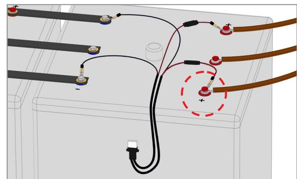
For batteries with four poles, please connect the BACS measuring cable to all poles.
