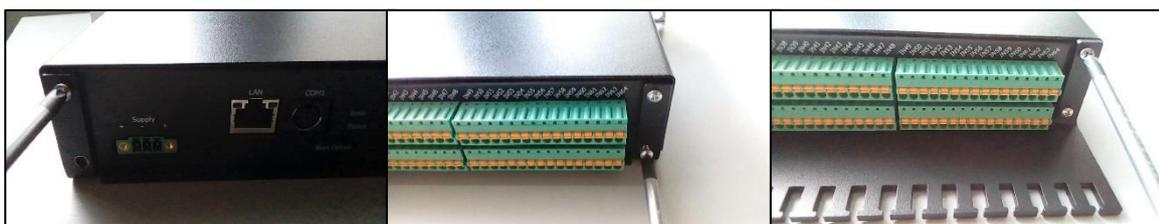
Remove the screws to release and place the cable comb. Then reattach cable comb with the screws.
