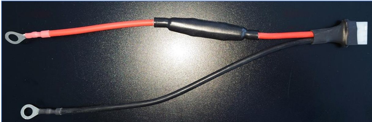
The picture shows a typical halogen free BACS BC5 measuring cable. The gas-tight sealing of the 1000V fuse is clearly visible. The gas-tight sealing prevents that hydrogen emitted during the charging process can be ignited.
