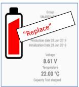
With the SMARTBATTERY COMPANION APP, you can define threshold values that are individually adapted to the location and contractual conditions, which can be used to immediately determine whether potential operation outside of the specifications has occurred during regular on-site maintenance.
