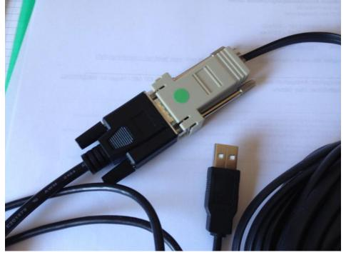
To get a permanent joint between the CS121\_AUX\_Adapter and the IBM UPS – RS232 Converter, please use the provided union nut:
