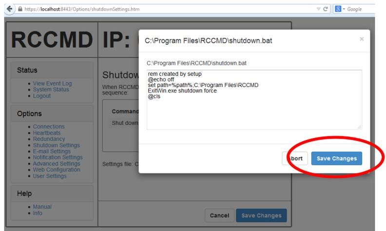
Fig. 29: RCCMD WebInterface Configurator – Shutdown Settings – Edit File
