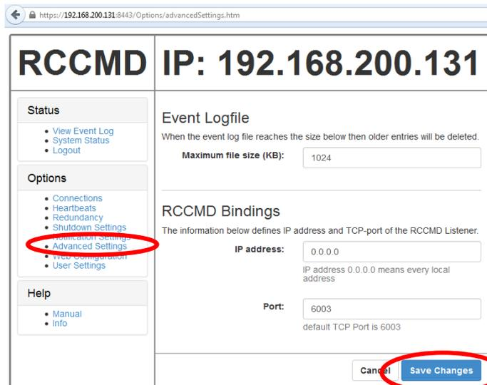
Fig. 104: RCCMD WebInterface – Advanced Setting
