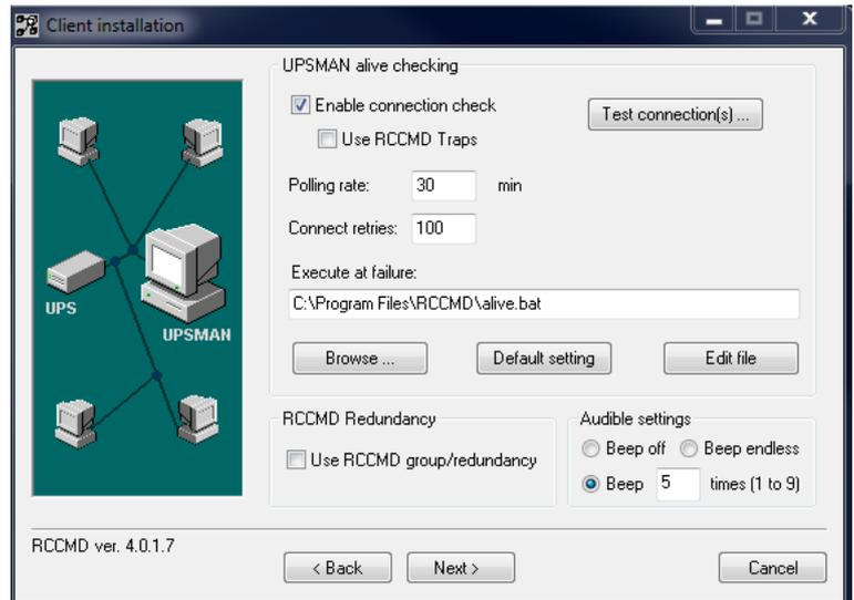
Fig. 63: UPSMAN Alive Checking / Redundancy Window
