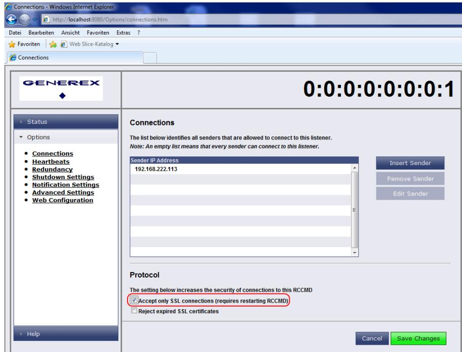
Fig. 46: RCCMD Web Configurator - SSL Konfiguration
