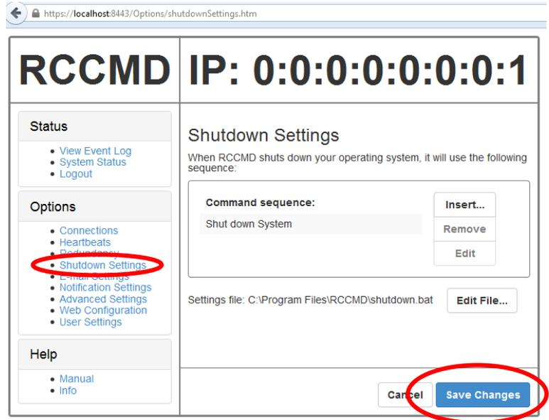
Fig. 28: RCCMD WebInterface Configurator – Shutdown Setting
