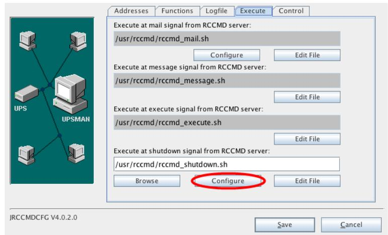
Fig. 124: Configuration – RCCMD Shutdown.sh
