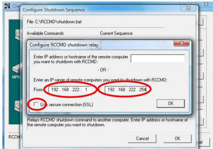
Fig. 74: RCCMD Configuration IP Address Range
