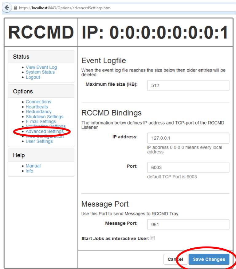
Fig. 32: RCCMD WebInterface Configurator – Advanced Settings
