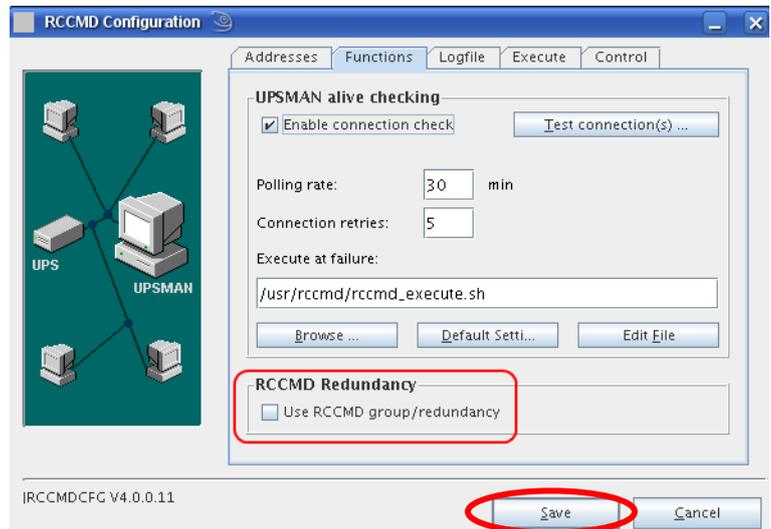
Fig. 120: Configuration – RCCMD Redundancy
