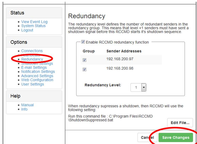
Fig. 27: RCCMD WebInterface Configurator – Redundancy
