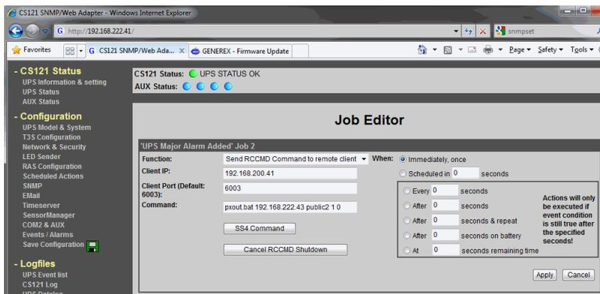
Fig. 188: CS121/CS141 Configuration for such a relay command
