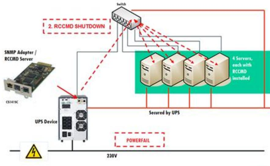
Fig. 1: Schema RCCMD
