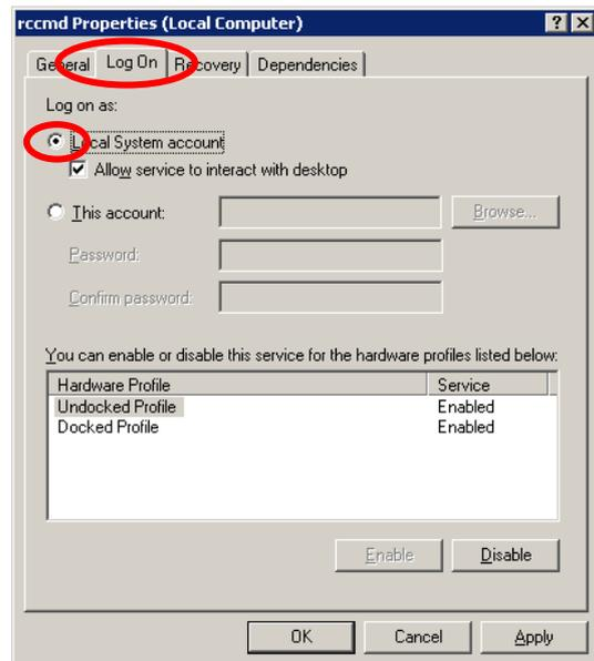
Fig. 48: RCCMD Properties Log On Window
