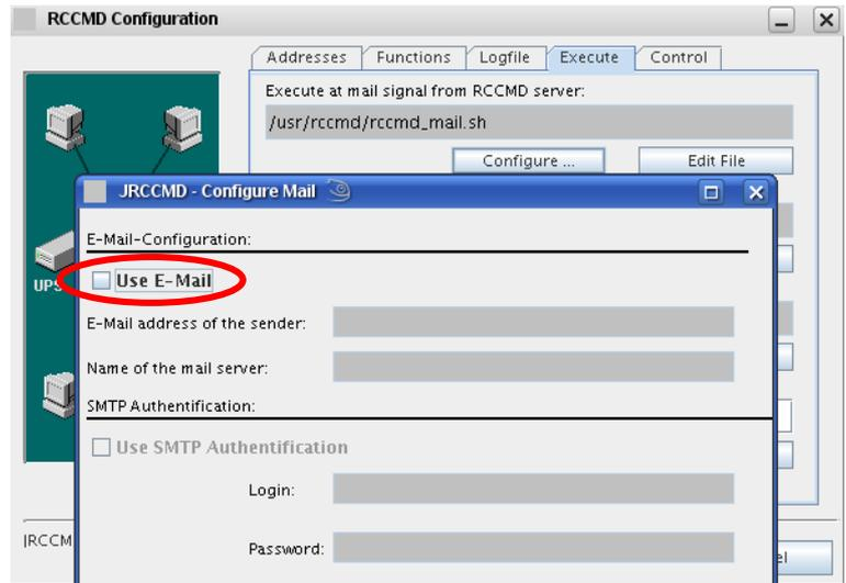
Fig. 123: Konfiguration – RCCMD Configure Email
