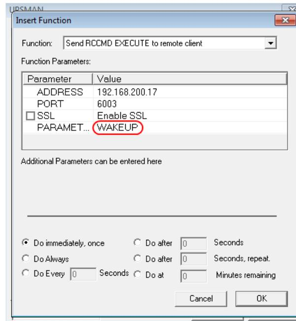
Fig. 41: CS121/CS141 Configuration “WAKEUP” Command
