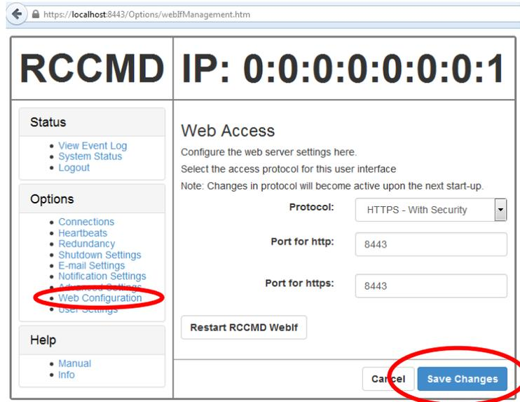
Fig. 33: RCCMD WebInterface Configurator – Web Configuration
