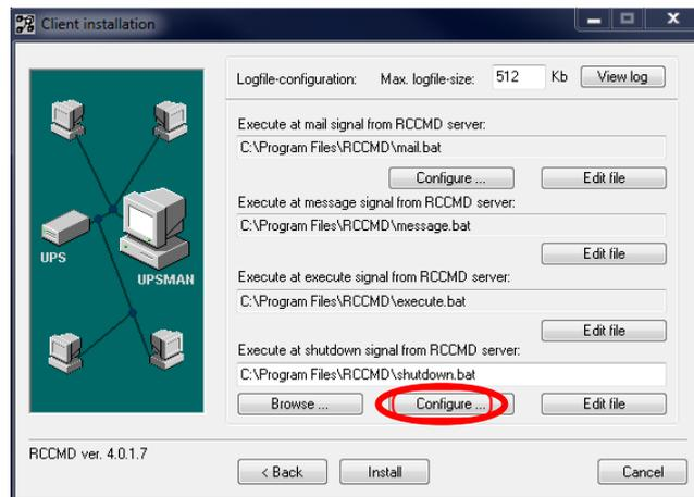
Fig. 72: RCCMD Client Shutdown Configuration
