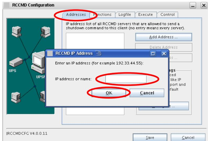
Fig. 118: Configuration – RCCMD Sender IP Address
