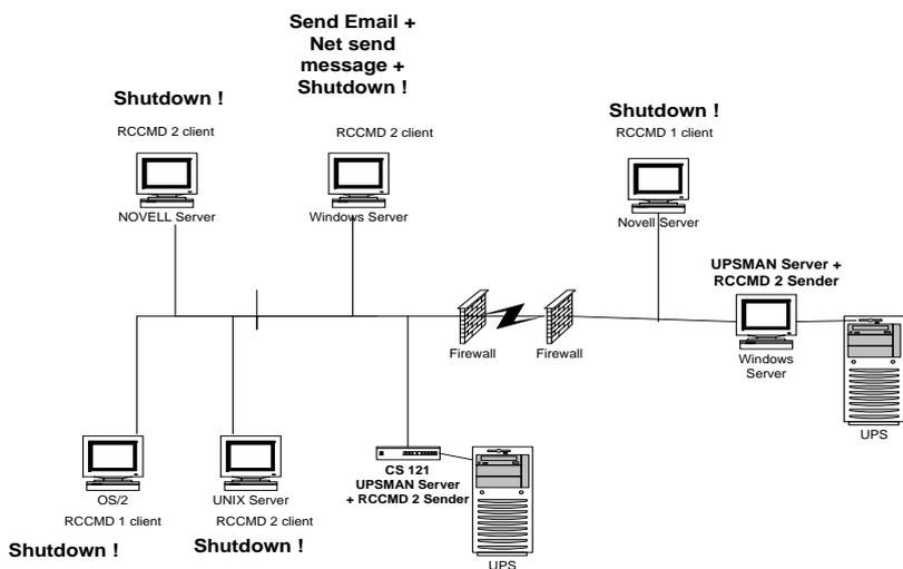
Fig. 2: RCCMD and UPSMAN in a network environment
