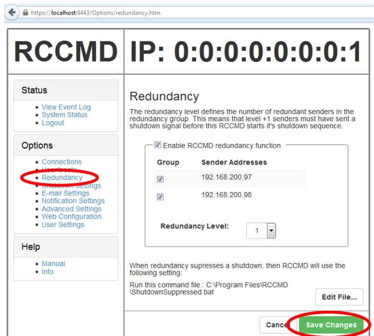
Fig. 101: RCCMD WebInterface – Redundancy
