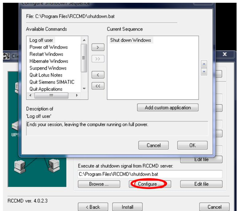
Fig. 70: RCCMD Shutdown Sequenz Configuration
