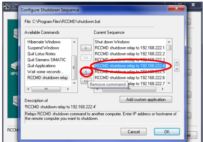
Fig. 75: RCCMD Shutdown Relay Removal
