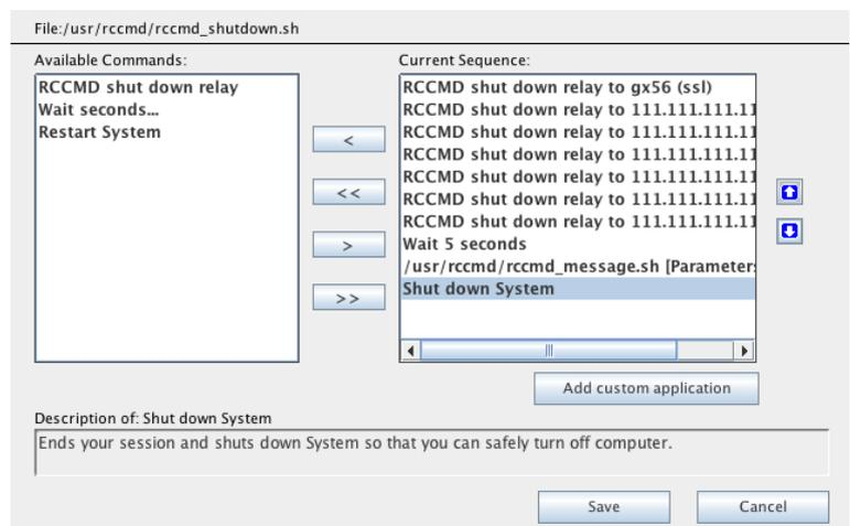
Fig. 125: Konfiguration – RCCMD Shutdown Sequenz
