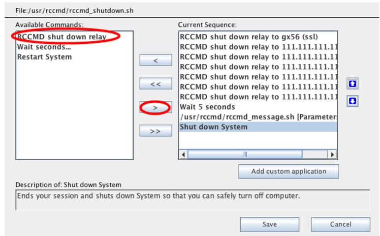
Fig. 128: Configuration – RCCMD Shutdown Sequenz
