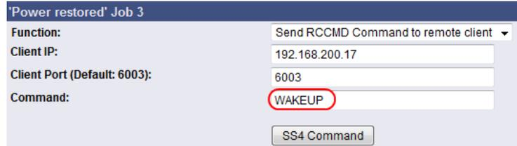
Fig. 40: CS121/CS141 Configuration “WAKEUP” Command
