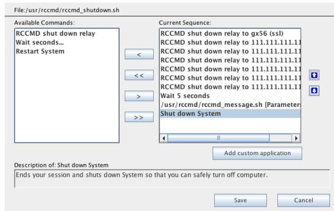
Fig. 182: Configuration – RCCMD Shutdown Sequenz
