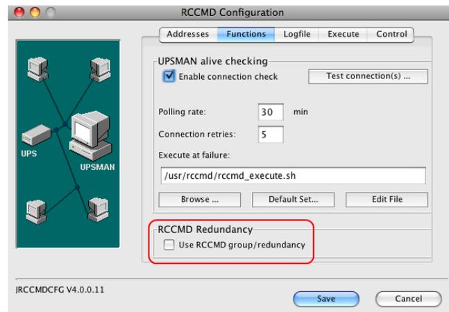
Fig. 177: RCCMD Redundancy
