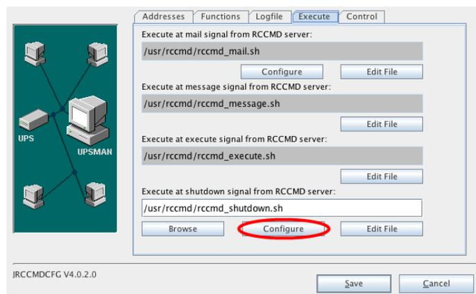
Fig. 181: Configuration – RCCMD Shutdown.sh
