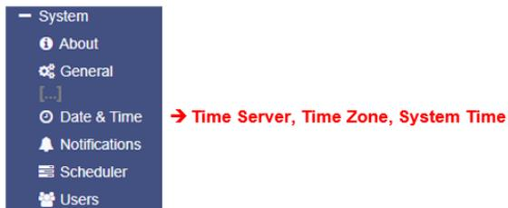
For some system-critical settings such as event logs or recurring tasks, an exact time specification is necessary. For this reason, the CS141 has its own system clock and the option of querying external NTP servers.
