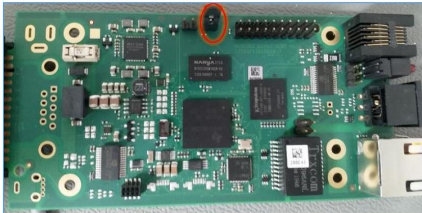
When the jumper is set and the adapter boots, you can identify the rescue system by the firmware version in the About screen - behind the firmware version you will find the word (RESCUE).
