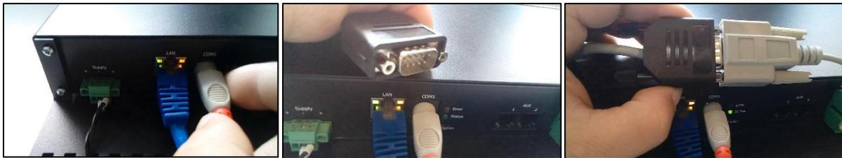
To ensure correct hold, place the screw nuts included in delivery between the two small locking devices.
